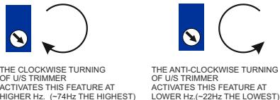
THE CLOCKWISE TURNING OF U/S TRIMMER ACTIVATES THIS FEATURE AT HIGHER Hz. (~74Hz THE HIGHEST)
