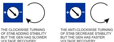
THE CLOCKWISE TURNING OF STAB ADDING STABILITY BUT THE GEN HAS SLOWER VOLTAGE RECOVERY.
